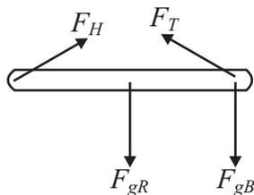
Note:  $F_{gR}$  is shown as acting at the center of mass of the rod.
