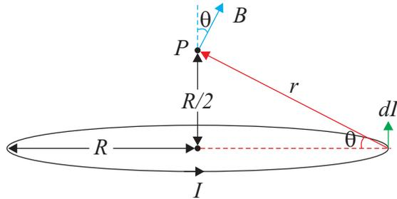
The current segment is tangent to and in the plane of the loop.
